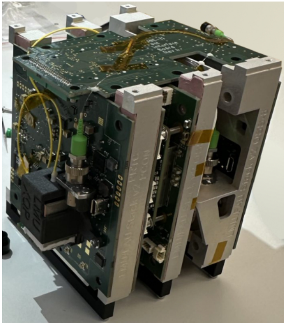
FIG. 1. The quantum payload stack of the QUBE-II mission during payload integration. A fast interface board at the top connects the payloads electrically.
